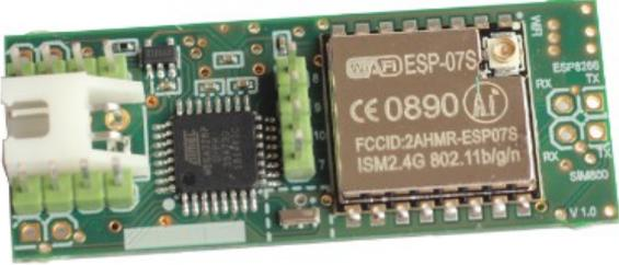
A green printed circuit board (PCB) for the Bike Bean project. It features a central ESP-07S module with a SIM card slot, various electronic components, and a white connector on the left side. The board is labeled with 'ESP-07S', 'CE 0890', 'FCCID:2AHMR-ESP07S', 'ISM2.4G 802.11b/g/n', and 'V 1.0'. | 1 x Bike Bean Platine                                              |
